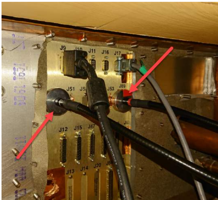
The optical couplers mounted in a filter plate (viewed from the operator room of the PET/MR).
